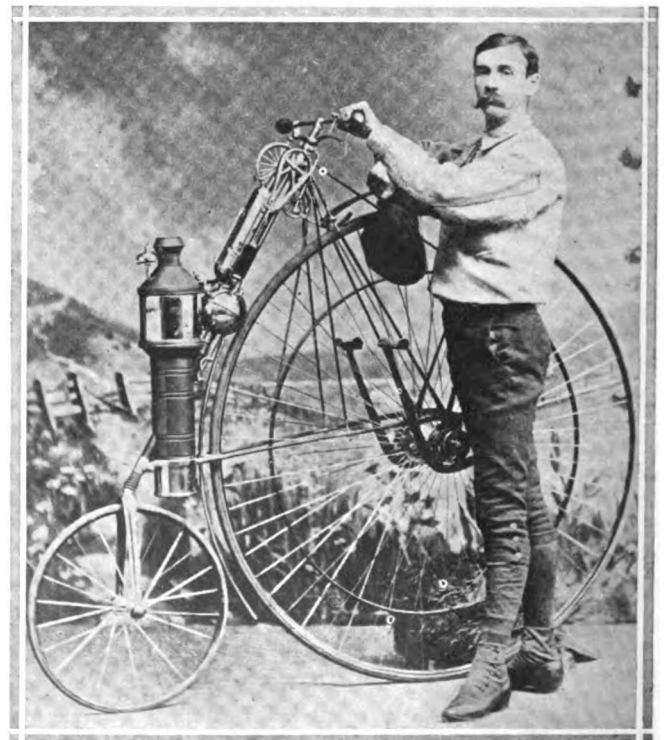
Lucius D. Copeland and his first successful steam motor, which is shown fitted to a Star bicycle of the vintage of 1884
